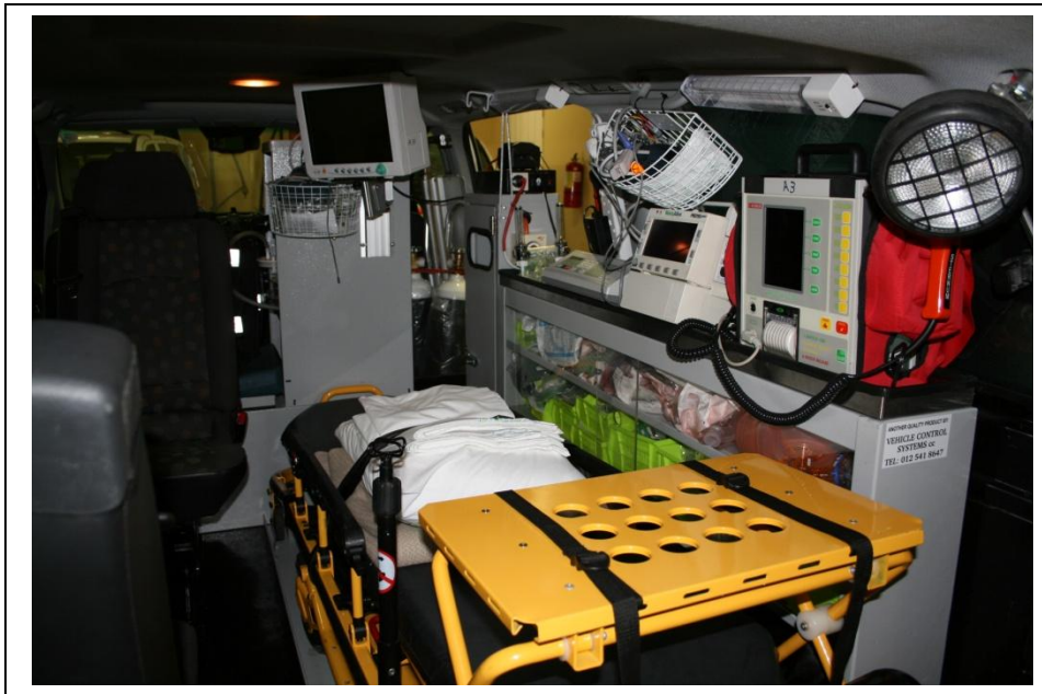
Long distance MICU ambulance configuration
